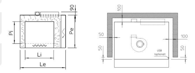
Maintenance is performed by moving the oven forward using the standard wheels. Alternatively, keep 600 mm of free space on the right side for the electric panel and 600 mm on the rear for the steamer. In addition, a free space of 50 mm deep is required for the maintenance of the computer touch and of the door opening system, for the reset of the safety thermostat and for the possible access to the USB socket (optional).
